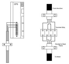
Power Block Clamp and Terminal Clamp
