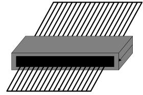
Flat cable clamp used with ribbon cable
