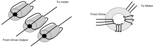
Common mode currents occur from noise spikes created by the PWM switching frequency of the drive. The use of a ferrite or iron-powder core toroid, as shown in the figure above, places common mode impedance in the line between the motor and the drive. The use of a common mode choke on the motor leads may increase signal integrity of encoder outputs and associated I/O signals. The following is a list of toroidal and ferrite cores that can be used to make common mode chokes:
